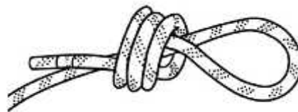
c) Scaffold knot with triple twist: loose
